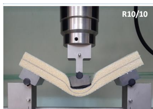
Fig. 4: Force-deflection behaviors of the specimens against bending
