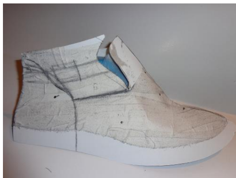
Fig3.a: Fixing the basic design on the last
