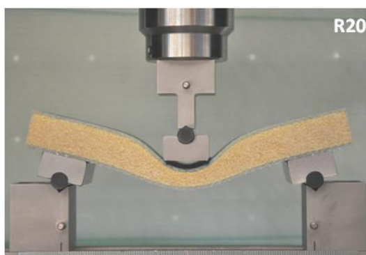
Fig. 4: Force-deflection behaviors of the specimens against bending
